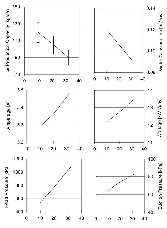
The horizontal axis shows the ambient temperature. It refers to the data of at/wt=10/10,21/15,32/21,40/35.
