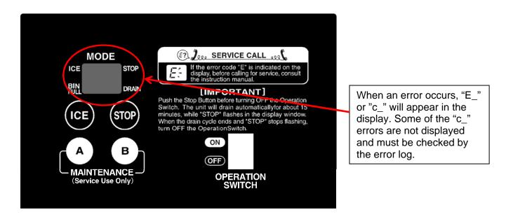
When an operational error occurs, "E\_" will appear and blink in the display on the operation board, and the icemaker will stop. When a service call is received, ask the user to check which error code is in the display. Then, see the error code table in "7. ERROR CODES" to locate the cause.
