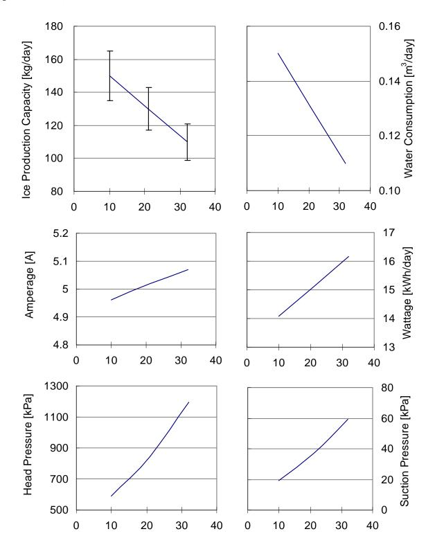
The horizontal axis shows the ambient temperature. It refers to the data of at/wt=10/10,21/15,32/21,40/35.
